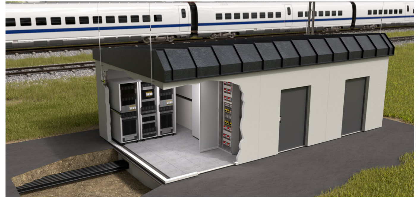
The track field concentrator is the link between the technology locations and the track field elements.
